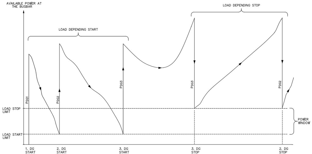
**A load-dependent start/stop example stated with 3 generator sets**
