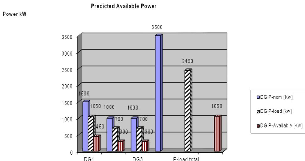
The calculated **predicted available power** is compared with the programmed load-depending start/stop limits in order to generate the PMS start/stop commands.
