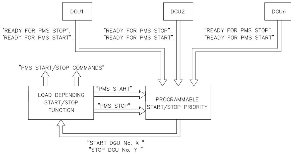
**Operating principle for determination of the start/stop priority**
